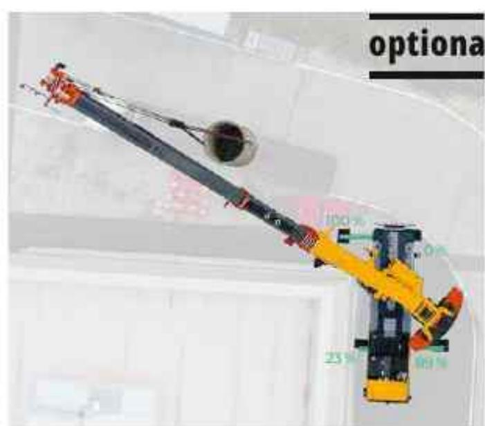
• Variables Ausfahren der Schiebebeine variable extension of outriggers to any position
